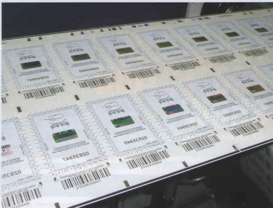
Holograms are applied to vehicle tax vignettes as a security device - note the mirror number which displays through the windshield
